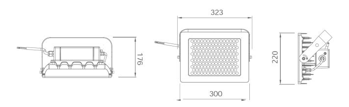
The solid die-cast aluminum housing is equipped with a rotatable bracket made of stainless steel.
